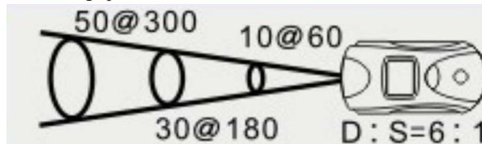
3. Measuring radius: make sure the surface to be measured is larger than measuring spot. If the target is small, place the thermometer closer to the target. For an accurate reading, make sure the target surface is two times larger than measuring spot.
